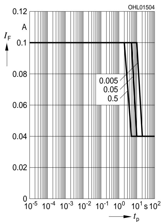
**Zulässige Impulsbelastbarkeit  $I_F = f(t_p)$** **Permissible Pulse Handling Capability**Duty cycle  $D$  = parameter,  $T_A = 85$  °C
